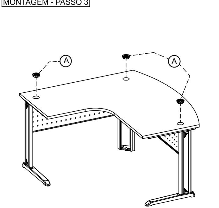
PARA FINALIZAR APÓS MONTAGEM COMPLETA DA MESA INSERIR O PASSA FIO (A).
