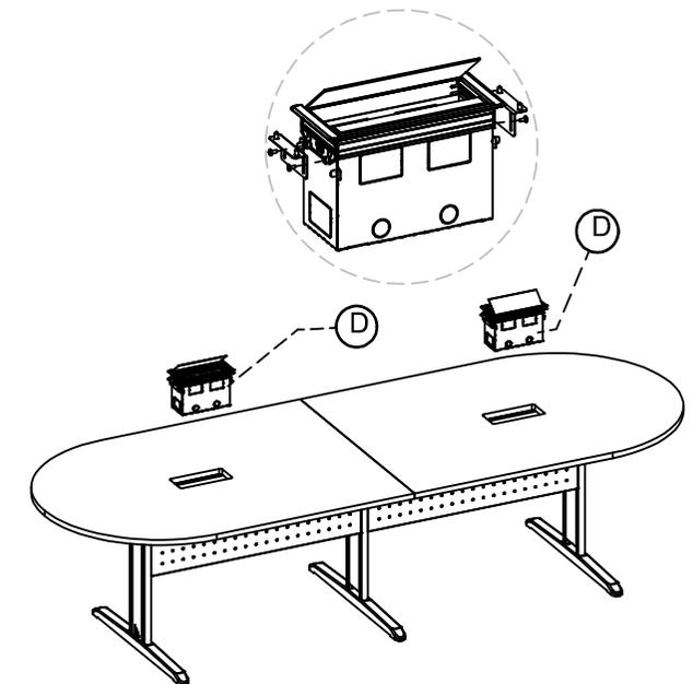
PARA FINALIZAR A MONTAGEM, PEGUE A CAIXA BASIC (D) E DESTAQUE AS ABAS LATERAIS CONFORME DETALHE 4, PARA QUE A MESMA POSSA SER FIXADA NA MESA.
